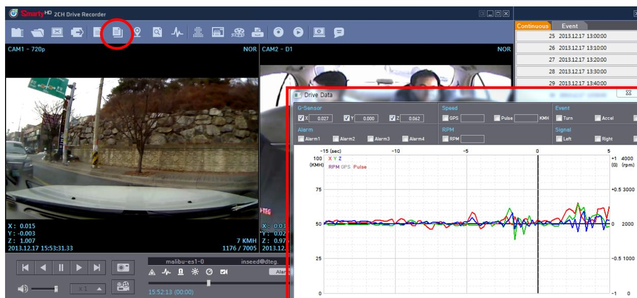
The default setting only displays the G-sensor graphs but other information may be added by checking the boxes in the upper part of the screen as below.
