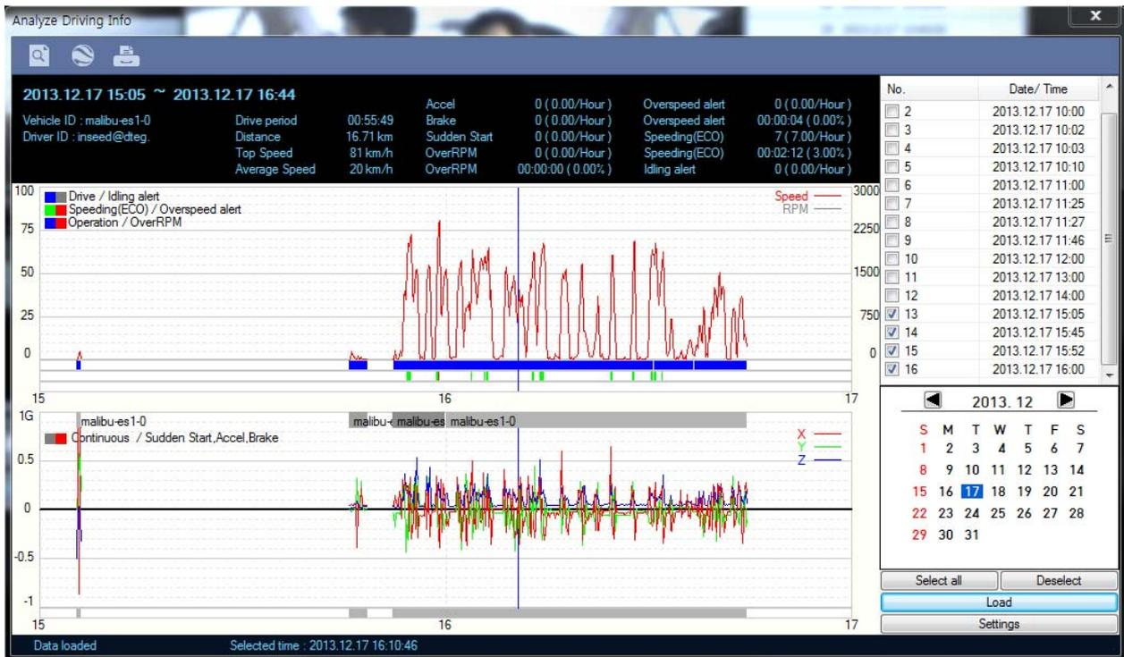
A summary of information can be found on the top including vehicle ID; Driver ID; Drive period; Distance; and number of over-accelerations, over-decelerations, sharp turns, over-speeding, over-RPMs that exceeded the pre-set limit.
